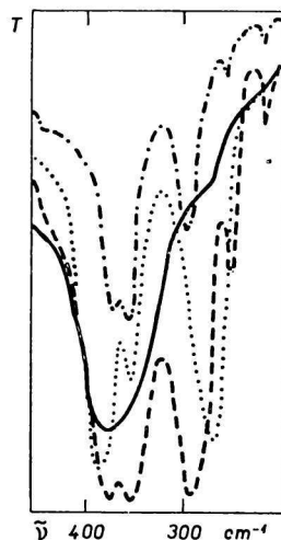
Fig. 4. Far infrared spectra of \text{TiCl}_3 \cdot 3\text{THF} , \text{TiCl}_3 \cdot 2\text{THF} , \text{TiCl}_3 \cdot 2\text{THF} \cdot \text{C}_6\text{H}_6 , and \text{TiCl}_3 \cdot \text{THF} .
