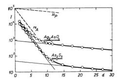
The experimental points are marked by circles. The analysis of both experimental curves is also shown in Fig. 1; the dashed straight line designates the theoretical decay curve for the decay of the radionuclides <sup>32</sup>P and <sup>76</sup>As.
