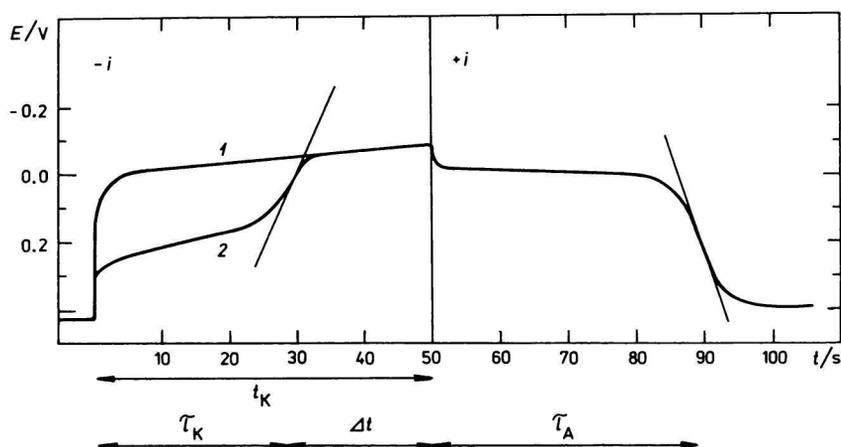
Fig. 1. Chronopotentiometric record of deposition and dissolution of aluminium (1) and lead (2). Current density pulse:  $0.59 \text{ mA cm}^{-2}$ ;  $c(\text{AlBr}_3)$ :  $1.86 \text{ mol dm}^{-3}$ ;  $c(\text{PbBr}_2)$ :  $3.13 \times 10^{-3} \text{ mol dm}^{-3}$ .
