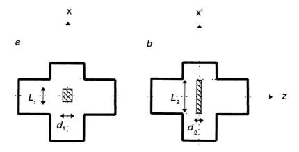
Fig. 1. Schematic diagram of the cross-section of the microwave rectangular cavity, in the centre of which the solid state cylindrical samples with identical volume, but different shape were inserted. (For more details see text.)
