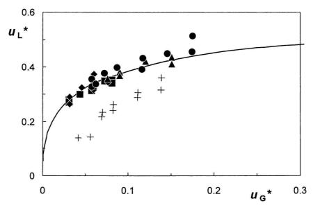
Fig. 3. Dimensionless superficial velocity of liquid as a function of gas superficial velocity for particular values H. The values are normalized employing  $\zeta = 4.5$ .  $\blacksquare H = 1525$  mm;  $\blacklozenge H = 1471$  mm;  $\blacktriangle H = 1417$  mm;  $\blacklozenge H = 1307$  mm; + H = 1180 mm; --B = 0.005.
