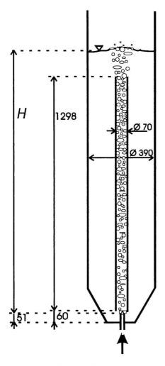
Fig. 1. Laboratory model 1 12 of the pachuca (dimensions/mm).
