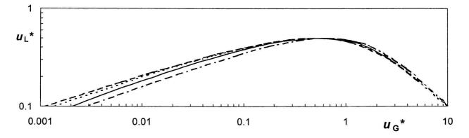
Fig. 2. Dimensionless superficial velocity of liquid as a function of gas superficial velocity for particular values of the parameter B. ----- B = 0.1; ---- B = 0.001; ---- B = 0.001; ---- B = 0.001.
