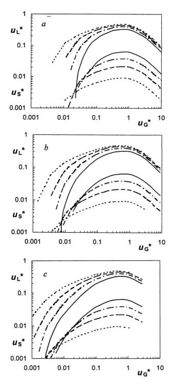
Fig. 4. Dimensionless superficial velocities of liquid and solid as a function of gas flow rate for s = 2.75. Three plots are for different B, a) B = 0.01, b) B = 0.001, c) B =0.0001. Upper group of curves for different X belongs to  $u_{\rm L}^*$ , lower group belongs to  $u_{\rm S}^*$ .---- X = 0.02; ----X = 0.05; ---- X = 0.10; — X = 0.20.
